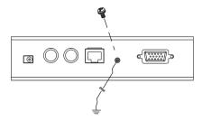
2. Make sure that the computer that the CE252L connects to and the monitor that the CE252R connects to are properly grounded.
