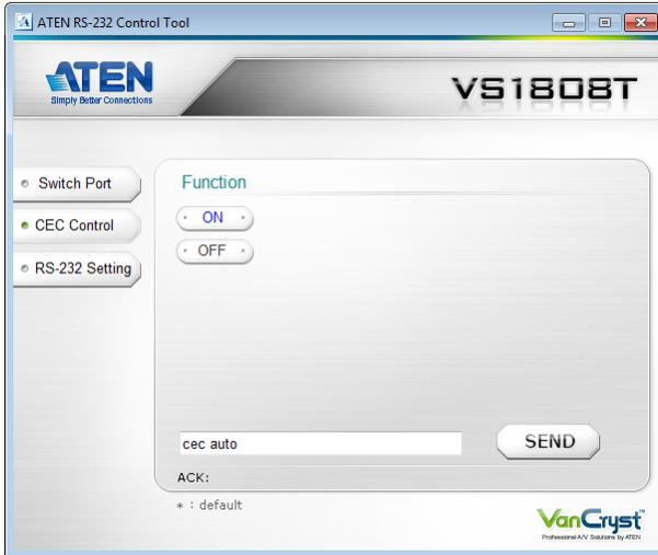
The CEC Control page is used to enable or disable the CEC Control feature. The default setting for the CEC Control is off.
