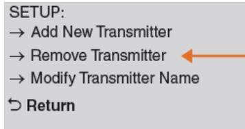
4. Use the **Up / Down** buttons to select the transmitter to be removed and then press **OK**.
